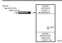
Fig. 73. Setup - Outputs - Floating Relay - Derivative.
