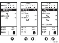
Fig. 21. LCD Display - Home Screen Displaying Sensors, Mod Outputs, and Active Relays.
