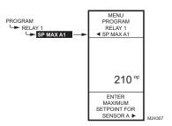
Fig. 28. Program - Sensor A Max. Setpoint.
