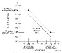
Fig. 25. Reset Curve for First Output with Setback Offset.
