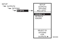
Fig. 66. Setup - Outputs - Options - DI Options.
