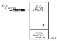
Fig. 62. Setup - Outputs - Number of Relays.
