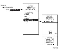
Fig. 53. Setup - Sensors - Sensor B - Throttling Range.
