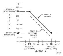
Fig. 36. Reset Curve with Offset for subsequent outputs.
