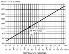
POSITIVE TEMPERATURE COEFFICIENT (PTC) OF 2.1 OHMS PER °F
