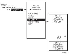
Fig. 52. Setup - Sensors - Sensor B - Hi/Low Limit.
