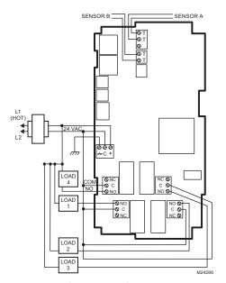
Fig. 9. Wiring for Four-stage Control – 24 Vac Input and 24 Vac Load.
