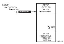
Fig. 59. Setup - Outputs - Mod Out - Derivative.
