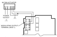
1 USE SEPARATE TRANSFORMER FOR T775R WHEN USING 24 VAC.
