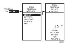
Fig. 35. Program - Setpoint Offset (subsequent outputs only).
