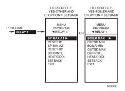
Fig. 27. Setpoint Values for Reset and Setback.
