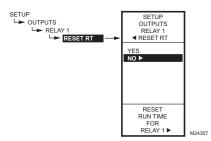
Fig. 76. Setup - Outputs - Relay - Reset Runtime.
