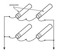
TO T775 CONNECTIONS (SENSOR A) OR (SENSOR B).
