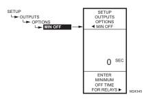
Fig. 65. Setup - Outputs - Options - Min Off Time.
