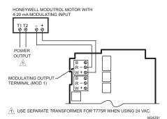
Fig. 14. Wiring for 4 to 20 mA Actuator.
