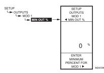
Fig. 57. Setup - Outputs - Mod Out - Minimum Output Percentage.
