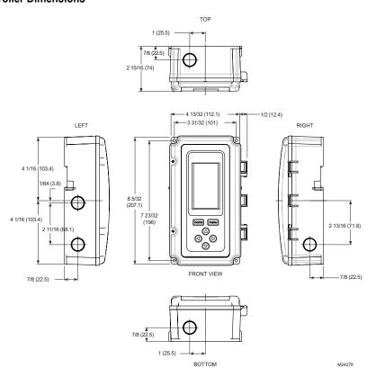
Fig. 1. T775R Dimensions in inches (mm).
